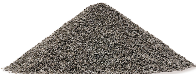
7.7 lbs granule loss per roll Acceptable per ASTM D4977
