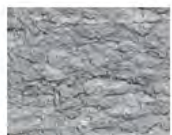
CSP 6 (Medium Scarification)
